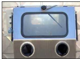
9. Water-jet cleaning 60 bar pressure
